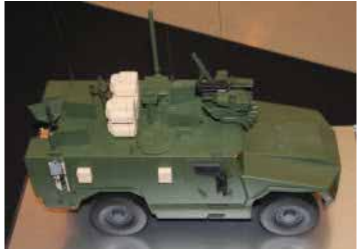
Scale model of VBMR-L fitted with roof-mounted remote weapon station, acoustic detection system, situational awareness system and counter-IED equipment
